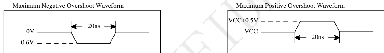
Figure 5-1 Maximum Overshoot Waveform
