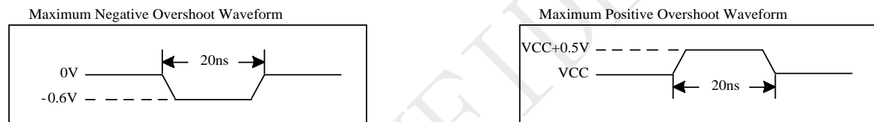
Figure 5-1 Maximum Overshoot Waveform
