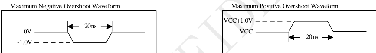
Figure 5-1 Maximum Overshoot Waveform
