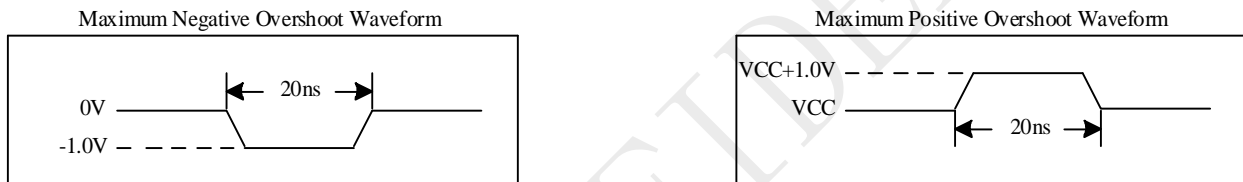
Figure 5-2 Input Test Waveforms and Measurement Level
