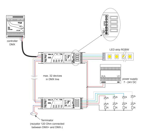
**Please note** that the driver is common anode type device. It is possible to connect lamps with 5-wires cable with a common "+" only.
