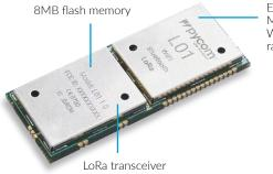
ESP32 Dual Core Microcontroller and WiFi/Bluetooth 4.2 radio
