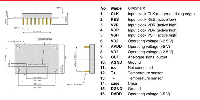
Note: Pixel 1 is nearest pin 1 of the device.
