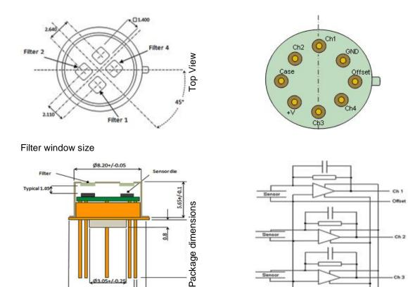
Note: Ensure that the sensor base is not in contact with the PCB in order to avoid shorts.
