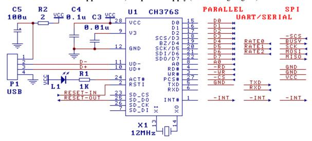
This is the 5V supply voltage of CH376 operation USB Flash Drive application circuit.
