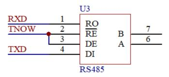
In the figure, TNOW is the switch pin, the TNOW pin can be used to control DE (send enable, high active) and RE# (receive enable, low active) pin of RS485 transceiver. RS485 transceiver should use the same power supply as VIO.
