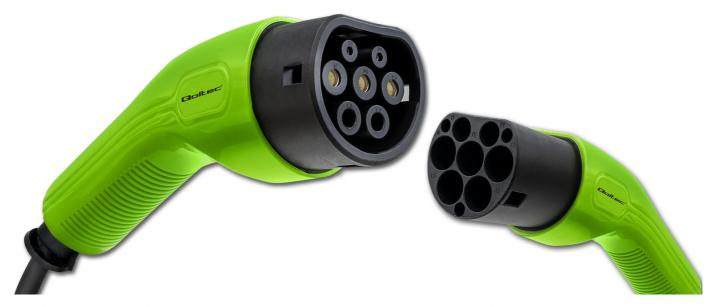
The cable has a Type 2 connector, which is now the official standard of the European Union and charges electric cars equipped with the corresponding charging socket. The Type 2 connector is 7 contacts, of which 3 contacts or 5 are for charging and 2 are for communication between the station and the car. Compatible with most electric cars sold in Europe.
