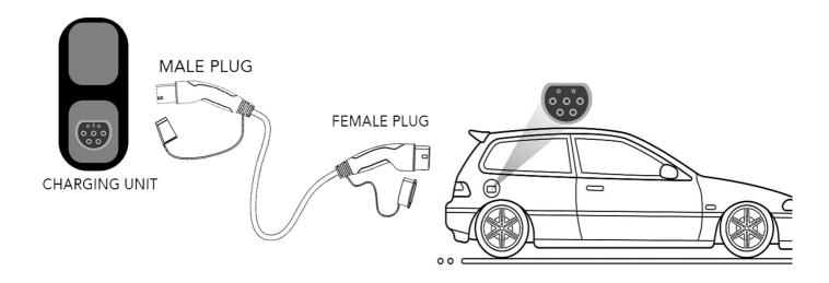
The cable has 2 male and 2 female connectors. The illustration above shows the correct way to connect the cable. The exceptional flexibility of the cable and the ergonomic shape of the pistol ensures complete comfort during daily use and storage of the cable. The mechanical life of the cable is ~ 10.000 connections, i.e. daily charging of your car for at least 25 years.
