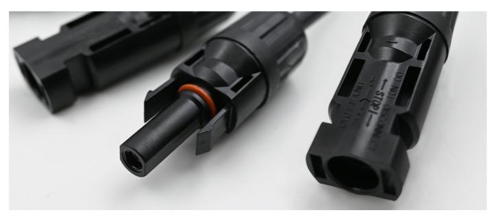
Qoltec brand connectors are used to **connect PV panels** in photovoltaic installations, using appropriate solar cables, also available in our offer. The set **includes a set of MC4 "+" and "-" connectors with pins**. Compatible with solar cables. They are designed to provide a safe and reliable electrical connection between PV modules. The product is designed for use with voltages up to 1000V.
