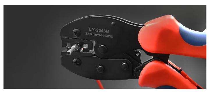
The practical crimping tool will allow the efficient and safe crimping of male and female solar connectors of type MC4. The crimper operates on the ratchet principle, has an automatic locking device and three working sockets for wires of 2.5 mm, 4.0 mm and 6.0 mm. The product is characterised by its robust construction made of high hardness steel and convenience of use.
