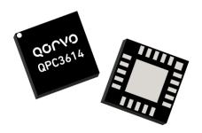
20 Pin 4.2 x 4.2mm QFN Package
