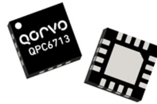
16 Pad 3.0 mm x 3.0 mm x 0.85 mm QFN package
