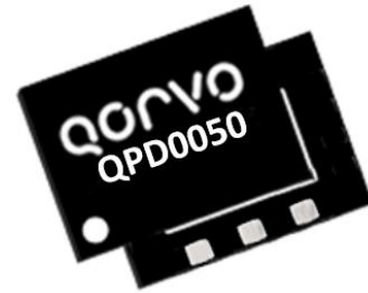
6 Pin 6.6 x 7.7 mm DFN Package
