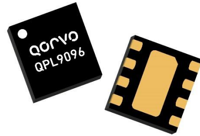
8 Pin 2X2 mm DFN Package
