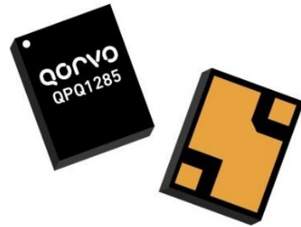
3 Pin 2 x 1.6 mm leadless SMT Package
