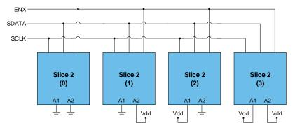
The Multi-Slice mode of operation allows up to four chips to be controlled from a common serial bus. The device address pins (15 and 16) ADD1 and ADD2 are used to set the address of each part.
