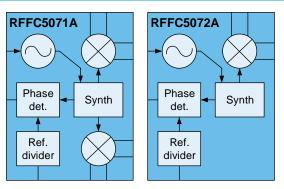
Functional Block Diagram - Top View
