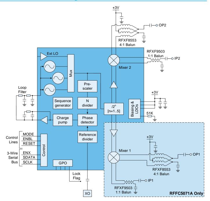
Note: Wideband transmission line transformer baluns shown above for operation to ~2.5 GHz. Substitute baluns for higher frequency applications as required.
