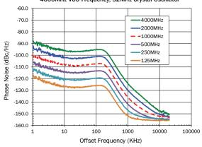
Synthesizer Phase Noise 5200MHz VCO Frequency, 52MHz Crystal Oscillator
