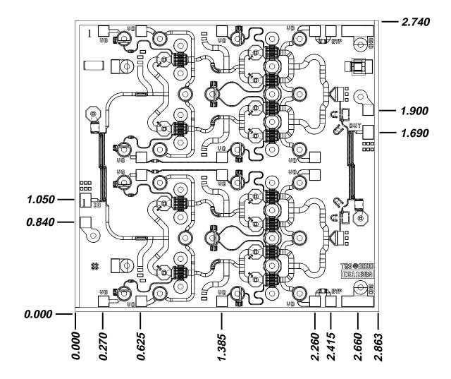
Dimensions in mm RF Pads: 130x100 μm DC Pads: 100x100 μm Die Area: 7.845 mm<sup>2</sup>
