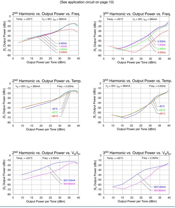
The plots reflect performance measured with an external coaxial bias tee and DC blocks
