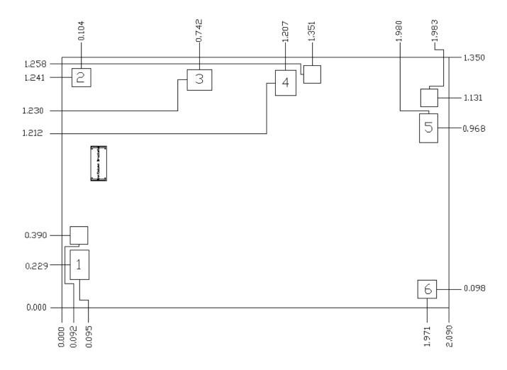
Unit: millimeters. Die thickness: 0.10, Die x, y size tolerance: +/- 0.050 Chip edge to bond pad dimensions are shown to center of pad. Ground is backside of die
