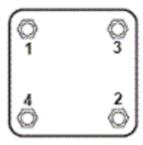
4. Apply no-flux solder to each pin of the TGA2590-CP. The component leads should be manually soldered, and the package cannot be subjected to conventional reflow processes. The use of no-clean solder to avoid washing after soldering is recommended.
