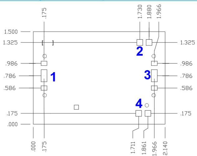
Unit: millimeters. Die thickness: 0.10, Die x, y size tolerance: +/- 0.050 Chip edge to bond pad dimensions are shown to center of pad. Ground is backside of die
