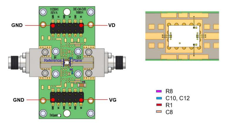
RF Layer is 0.008" thick Rogers Corp. RO4003C ( $\epsilon_r = 3.35$ ). Metal layers are 0.5 oz. copper. The microstrip line at the connector interface is optimized for the Southwest Microwave end launch connector 1092-01A-5. PCB level tuning at input side is recommended for optimal performance.
