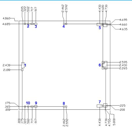
Dimensions are in mm Thickness: 0.10Die x, y size tolerance:  $\pm 0.050$ Ground is backside of die
