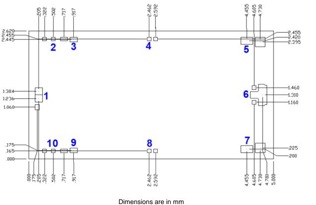
Dimensions are in mm Thickness: 0.10 Die x, y size tolerance: ± 0.050 Ground is backside of die
