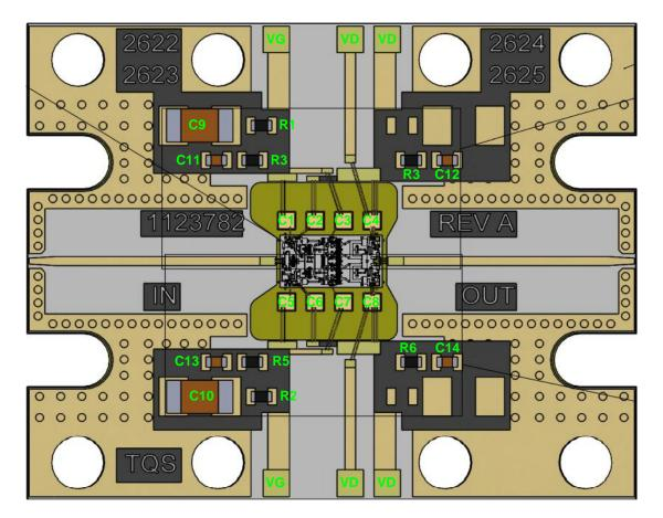
PCB is made from Rogers 4003C dielectric, .008 inch thick, 0.5 oz. copper both sides.
