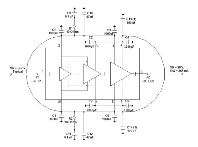
(1) Remove 100 uF capacitors (C13, C14) for pulsed operation.
