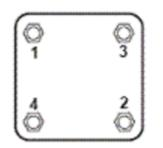
Apply no-flux solder to each pin of the TGA2625-CP. The component leads should be manually soldered, and the package cannot be subjected to conventional reflow processes. The use of no-clean solder to avoid washing after soldering is recommended.
