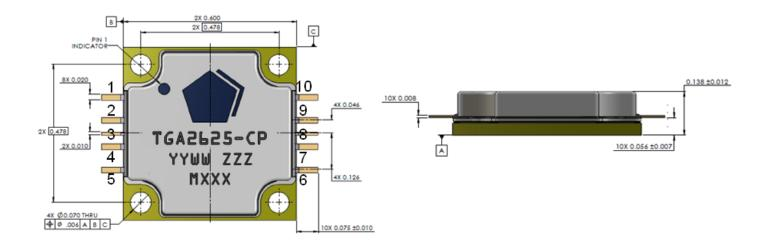
Units: inches Tolerances: unless specified  $x.xx = \pm 0.01$   $x.xxx = \pm 0.005$ Materials: Base: Copper Lid: Plastic All metalized features are gold plated Part is epoxy sealed Marking: 2625: Part number YY: Part Assembly year WW: Part Assembly week ZZZ: Serial Number MXXX: Batch ID
