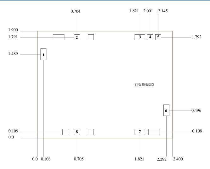
Unit: millimeters Thickness: 0.10
