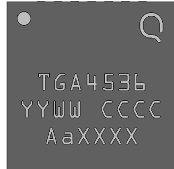
28 lead 5x5mm QFN package
