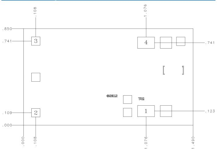
Unit: millimeters Thickness: 0.085 Die x, y size tolerance: +/- 0.050 Chip edge to bond pad dimensions are shown to center of pad Ground is backside of die
