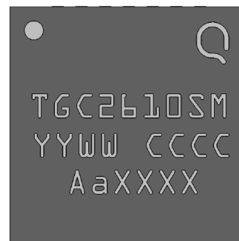
28-pin 5x5 mm QFN package
