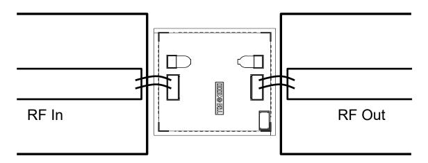
Note: RF Input and RF Output ports are not interchangeable.
