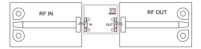
Note: RF Input and RF Output ports are not interchangeable.
