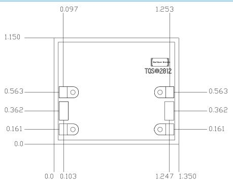
Unit: millimeters Thickness: 0.10
