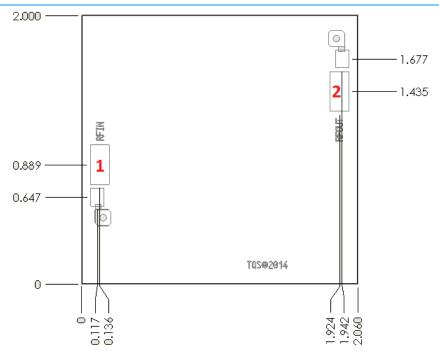
Unit: millimeters Thickness: 0.10
