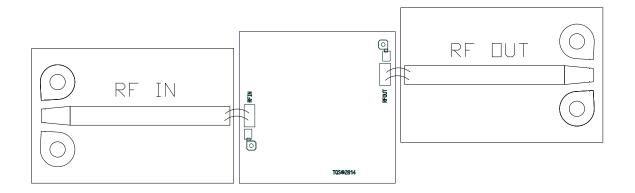
Note: RF Input and RF Output ports are not interchangeable.
