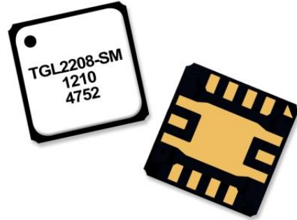
QFN 3 x 3 mm 14 L Package
