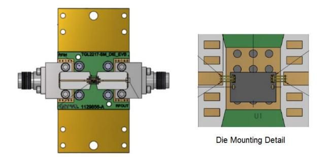
RF layer is 0.008" thick Rogers RO4003C,  $\varepsilon r$ = 3.38. Metal layers are 0.5-oz copper. The microstrip line taper at the connector interface is optimized for the Southwest Microwave end-launch connector 1092-01A-5.
