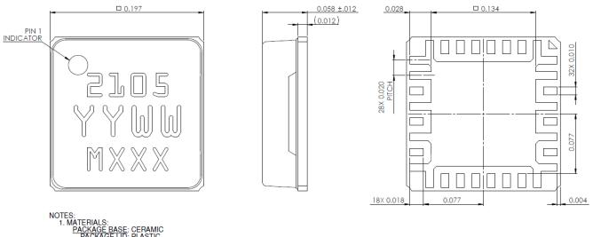
NOTES: 1. MATERIALS: PACKAGE BASE: CERAMIC PACKAGE LID: PLASTIC 2. PART IS EPOXIED SEALED. 3. PLATING: ALL METALLZED FEATURES ARE GOLD PLATED. 3. PART MARKING: 2105: PART NUMBER YY: PART ASSEMBLY YEAR WW: PART ASSEMBLY YEAR WW: PART ASSEMBLY WEEK MXXX: BATCH ID
