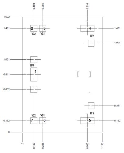
Unit: millimeters Thickness: 0.10
