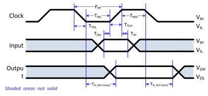
Figure 3-3 SPI slave timing
