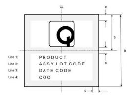
Figure 4-2 Package marking layout
