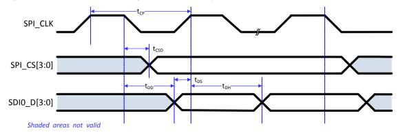
Figure 3-4 SPI master timing
