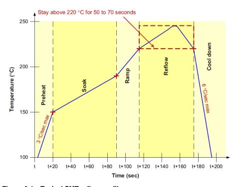
Figure 6-1 Typical SMT reflow profile
