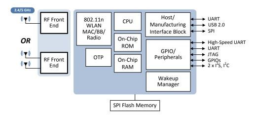
Figure 1-1 QCA4004 functional block diagram
