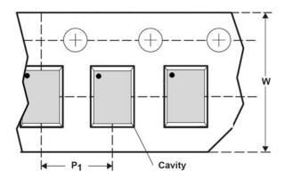
Figure 5-2 Part orientation in tape
