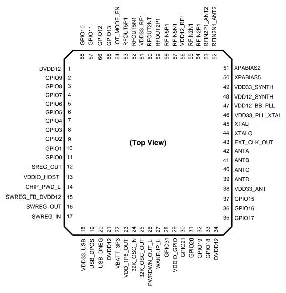
Figure 2-1 QCA4004 pin assignments (top view)
