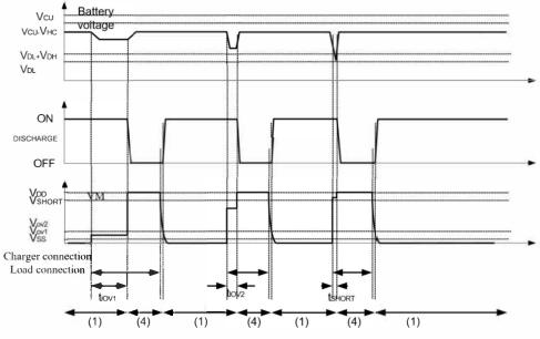
Figure 5-2 Overdischarge Current Detection
