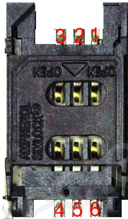
Figure 6: (U)SIM Card Interface
