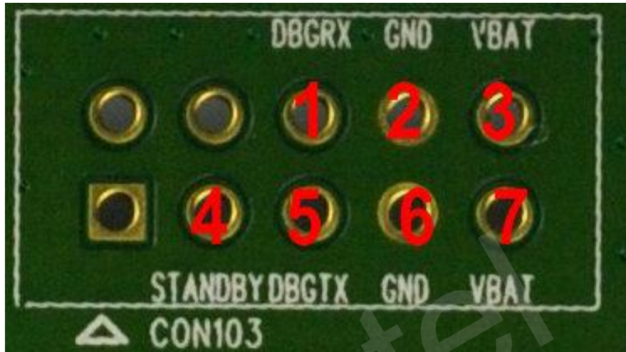
Figure 13: Test Points CON103
