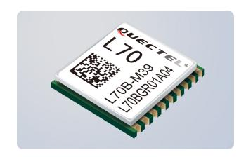
L70, an SMD type module, brings the high performance of MTK positioning engine to the industrial applications with compact profile, ultra low power consumption and fast positioning capability.
