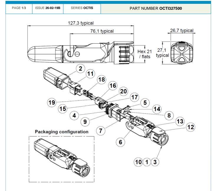
All dimensions are in mm. Tolerances according ISO 2768 m-H.
