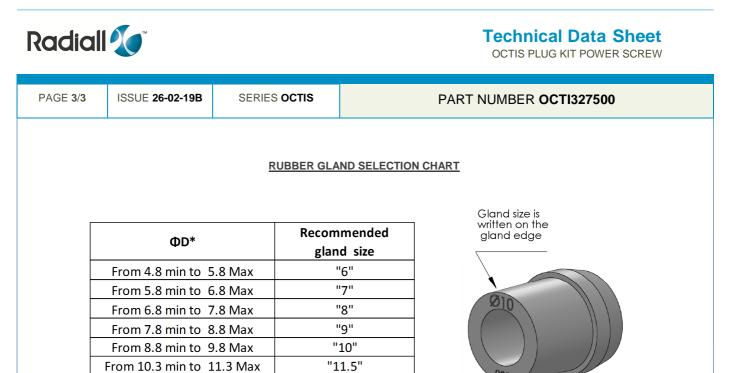
\*Cable diameter under the gland. If the cable has a sleeve, the diameter over the sleeve should be considered The tolerances of ΦD should be taken into account to make sure it is always within the specified range
