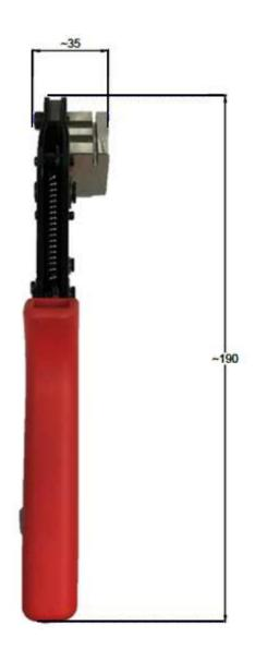
Manual crimping tool for power contacts. For stranded wires 1.5 mm² to 2.5 mm², AWG16 to AWG14. Suited for the following OCTIS plugs:
