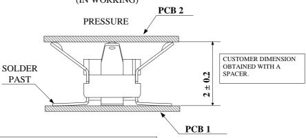
THE CONNECTOR IS NOT A SPACER, SO THE  $2\pm0.2$  DIMENSION A MUST BE ENSURED WITH AN ADDED PIECE PART SETTED 10 mm MAX.FAR FROM THE IMP CONNECTOR.
