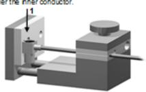
Place the connector into the tool. Place the gasket and the
