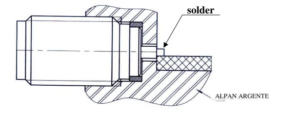
Assemble metal gasket onto connector. Screw the whole into the housing. Tighten the connector up to 210Ncm+or-10Ncm(use special tooling set RADIALL R282.341.002) Thus the connexion hermeticity is guaranteed at 10-8cc/sec. Then solder the pin on the track. Beware there is not too much solder.
