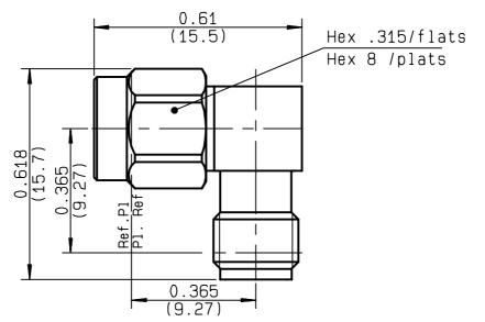
NOMINAL IMPEDANCE 50 **0-18** GHz FREQUENCY RANGE **-65/+165** °C TEMPERATURE RATING **1.10** + **.006** x F(GHz)Maxi V.S.W.R 0.07 √F(GHz) dB Maxi RF INSERTION LOSS 500 Veff Maxi **VOLTAGE RATING** DIELECTRIC WITHSTANDING VOLTAGE 1000 Veff Mini
