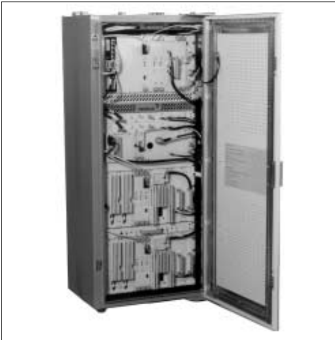
Base station of cellular network
