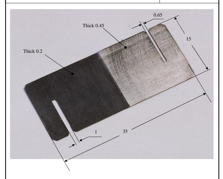
GAUGE FOR SEMI-RIGID CABLE TYPE .085 AND .141
